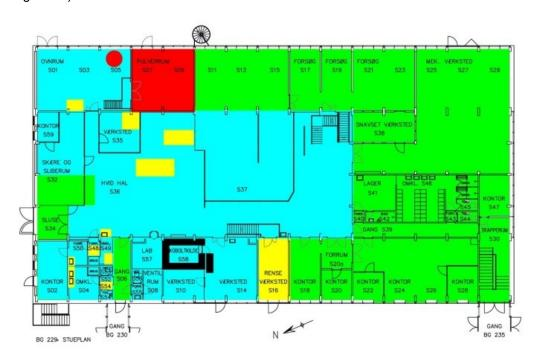
Figure 23: Classification by colours of the ground level before the start of decommissioning of the Fuel Fabrication Plant:
