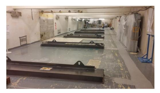
Figure 12: Dummy shutter housings with dummy shutters on the top surface of the row of hot cells, before modification.
