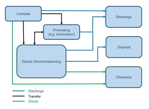
Figure 2: Generalised framework for management of radioactive waste in Denmark.
