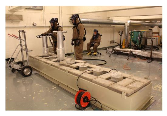
Figure 17: The complete setup of the steel grit blasting. The blowing nozzle is placed in the first hole and the camera in the third.
