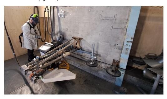
Figure 9: Testing of wire cutting
