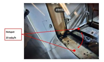
Figure 20: The hotspot was stuck under the door
