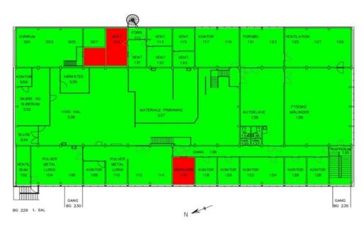
Figure 24: Classification by colours of the first floor level before the start of decommissioning of the Fuel Fabrication Plant:
