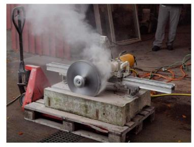
Figure 34: The milling tool in action
