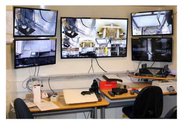
Figure 3: The control room in the basement, from where the equipment is operated. The screens show pictures from inside the reactor tank.
