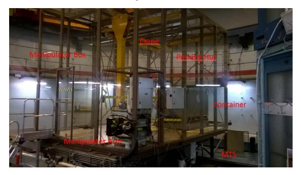
Figure 2: The Packing Hut and the Manipulator Box installed on the MTS on the reactor top.
