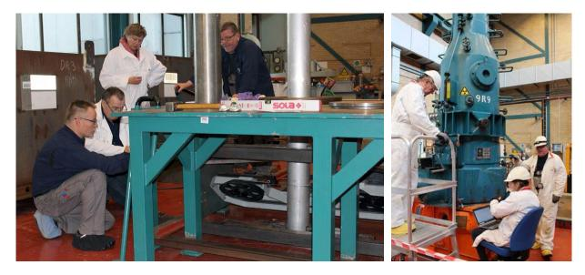
Figure 17: Horizontal saw (to be shielded with concrete blocks) on which the flask is going to be placed.
