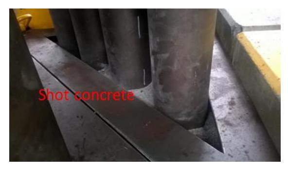
Figure 11: A corner container filled with fuel element plugs and shot concrete
