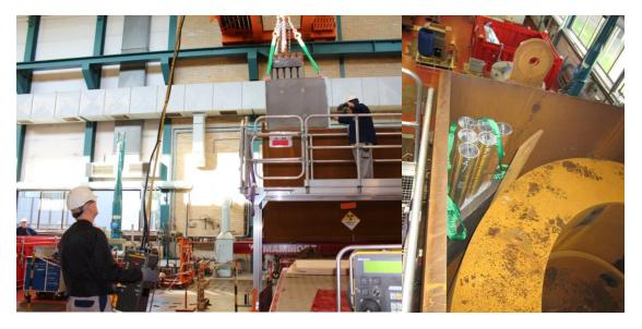
Figure 12: Loading a corner container with FE-plugs into a Jumbo container.
