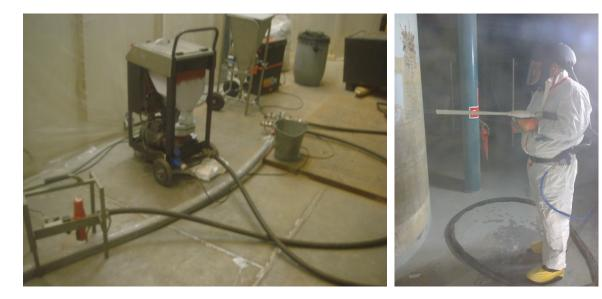
Figure 6: The CO2 ice blasting equipment
