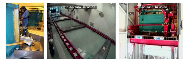
Figure 22: Circular saw for cutting the shutters.
